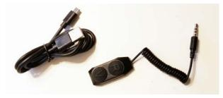
Your Omega sight comes with a remote control tether ("rat tail") accompanied by a small strip of Velcro adhesive for securing the remote in a convenient location. Simply plug the male end into the port located on the left side of the LCD Screen. There are two buttons on the remote. "R" button works the same as the "Power On/Off Button." "V" button starts and stops the video recording.
