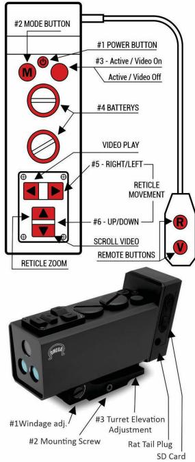
After setting Reticle in desired location. Make first Zero adjustments with #3 Turret (Elevation) and #1 Screw (Windage)
